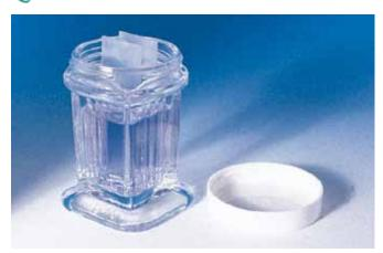
The screw cap is made of linerless white polypropylene that reduces solvent evaporation and spills during storage.
