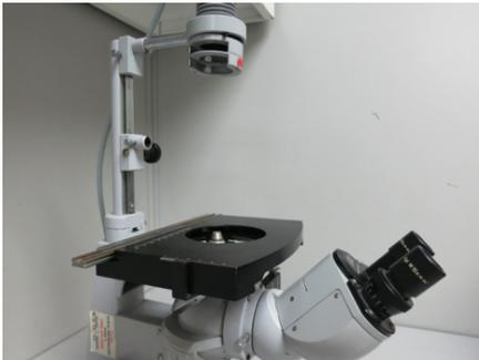
Begin by removing all stage accessories to provide a flat surface for the Cell Factory system to rest upon. If additional space is required, remove the light source.
