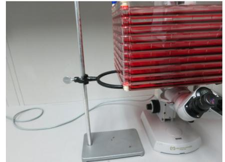
If the microscope stage is not capable of supporting the weight of the Cell Factory system, it is advisable to use an adjustable stand to carry some of the weight of the Cell Factory system.
