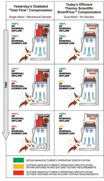
The advantage of the dual blower based Thermo Scientific SmartFlow design is shown here. As the filters load, the total flow compensating/ system with mechanical damper (left) results in increasingly divergent downflow and inflow, while the SmartFlow systems (right) remain within the validated performance envelope. Brown arrows and particulates depict the loss of product protection over time as the airflow balance changes due to filter loading.
